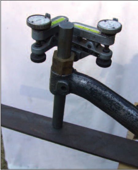
Photo 2 - Checking the castor angle with a special Dunlop gauge; this can also be used to check the kingpin inclination angle
