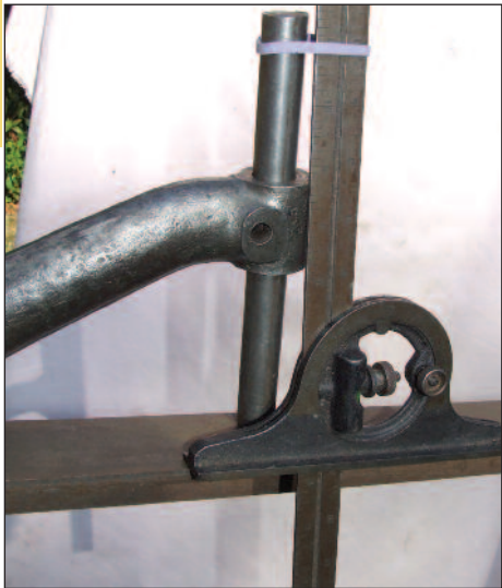
Photo 3 - Checking the kingpin inclination angle with a protractor; this can also be used to check the castor angle
